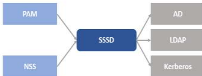
Figure 21: System Security Services Daemon Connectivity
